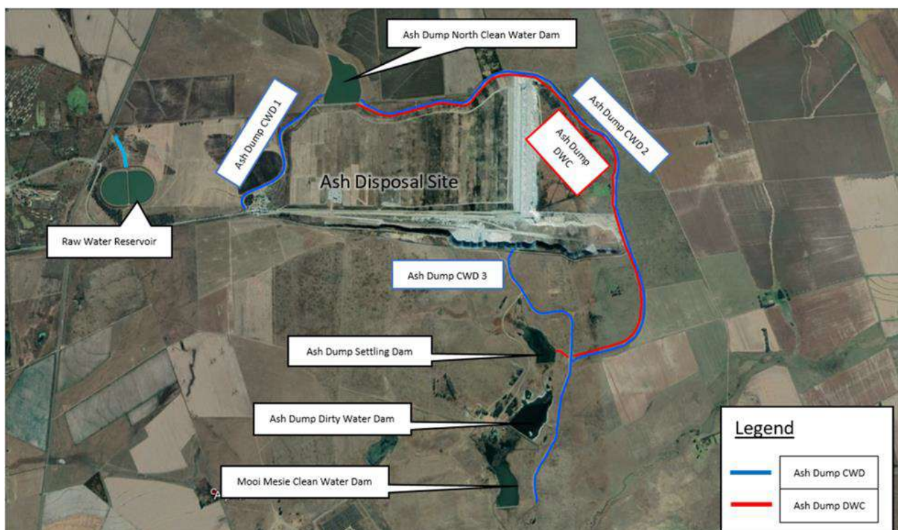
Figure 10: Ash Dump Open Drainage Channels Layout
