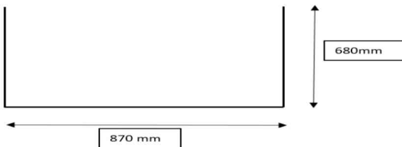
Figure 7: Cross-Section of the Concrete Pipe Trenches
